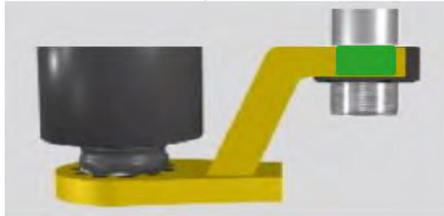
Figure 4.2.4-1: Correct Reaction Point
