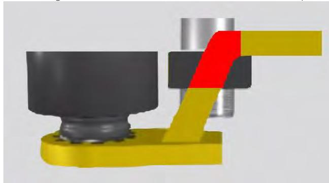
Figure 4.2.4-2: Incorrect Reaction Point
