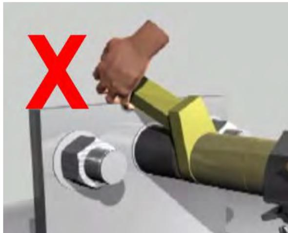
Figure 4.2.1-2: Incorrect Placement of Hand/Body Parts During Operation
