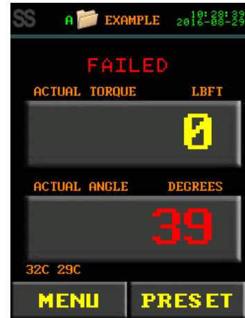
Figure 7.3-3: Failed Angle Cycle
