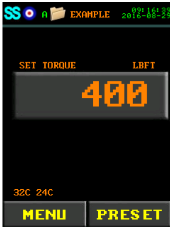
Figure 5.14-6: Main Screen, Point Cal Enabled
