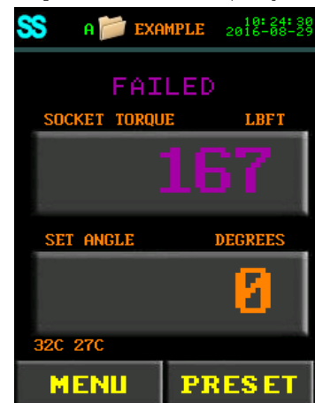
Figure 7.2-4: Failed Torque Cycle with Smart Socket Result
