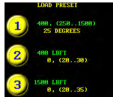
Figure 5.17-3: Presets 2 and 3 with Angle Limits in Brackets
