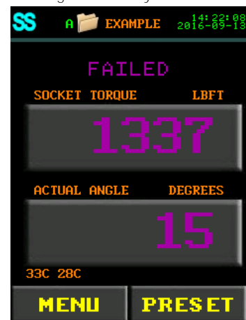
Figure 7.4-5: Failed Torque and Angle with Smart Socket
