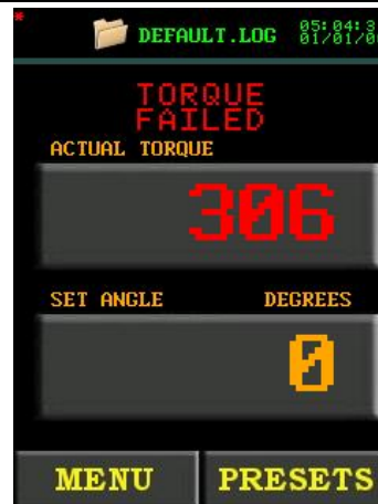
Figure 5.2-2: Failed Torque Cycle
