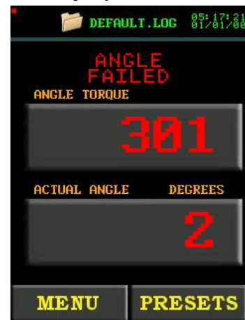
Figure 5.3-3: Failed Angle Cycle
