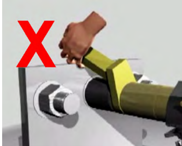
Figure 4.1.1-2: Incorrect Placement of Hand/Body Parts During Operation
