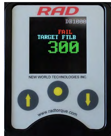
Figure 4.2-2: Failed Torque Cycle
